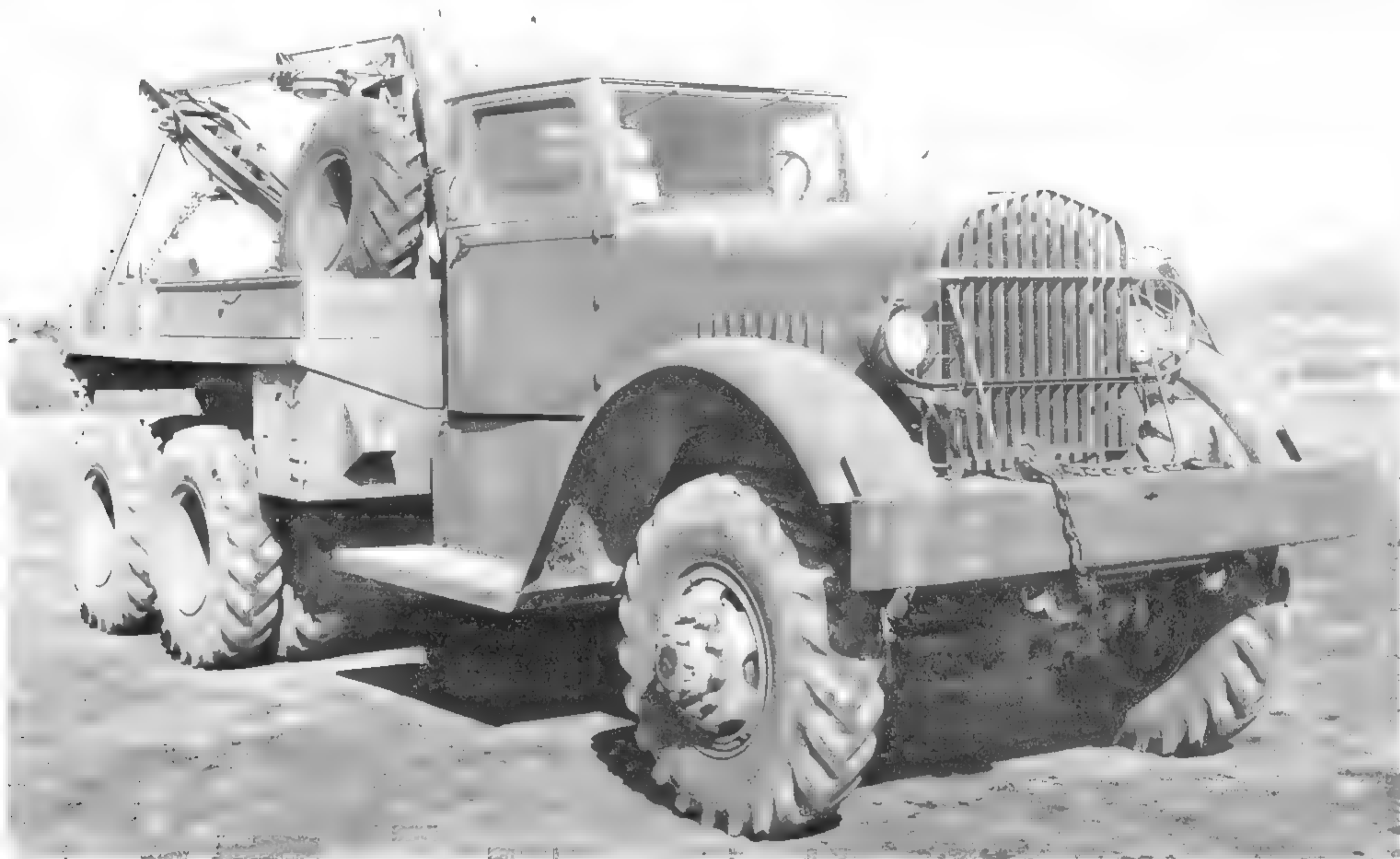
With the second series wreckers, the spare tires were relocated, with one behind the cab and the second on the crane tower. Ward LaFrance would retain this placement for the tires until the introduction of the fifth series wreckers. The long passenger's-side toolbox can also be seen in this February 1942 view. (NARA photo)
